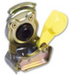
095.004 452 200 212 0 (0109 916) Automatic Coupling, Yellow M22x1.5
